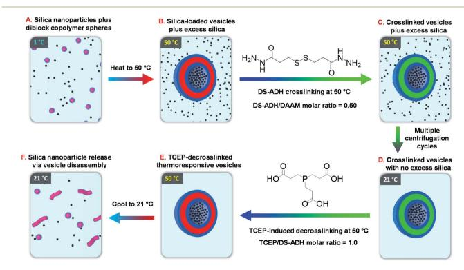
Fig. 1 Schematic overview of the six stages involved in the encapsulation and release of silica nanoparticles using a thermoresponsive 'shape-shifting' PDMAC<sub>56</sub>-P(HBA-stat-DAAM)<sub>254</sub> diblock copolymer.
