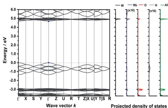
Fig. 5 Electronic band structure of  $\text{Rb}_3\text{WO}_4\text{H}$  and projected density of states (DFT-PBE0). The band paths in the reciprocal space have been determined by the Seek-path webservice.<sup>45</sup> The DOS of Rb and H are enhanced by a factor of ten for better visibility.
