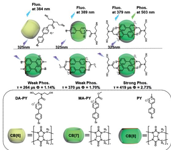
Fig. 10 Schematic illustration of the construction of "two-end blocked" pseudorotaxane based on CB[8] and DA-PY.
