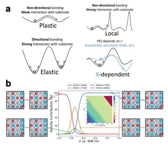
Fig. 3 (a) A depiction of the four classifications of fluxionality. (b) Isomer distribution of tungsten boride surface states for HER as a function of applied potential and pH.
