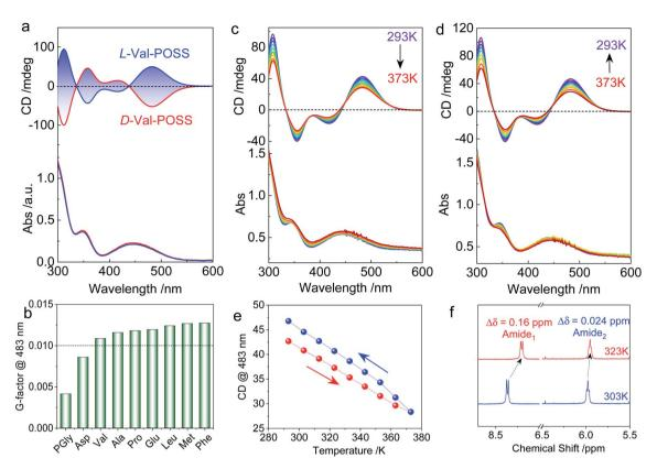
Fig. 3 (a) CD spectra of Val-POSS in CHCl<sub>3</sub> (1 mM) with different configurations. (b) Dissymmetry g-factors of different building units, "POSS" was omitted for clarity. (c-e) Temperature-variable CD spectra with heating and cooling processes of Val-POSS (1 mM in dioxane). (f) Partial <sup>1</sup>H NMR spectra of Val-POSS in CDCl<sub>3</sub> at different temperatures.
