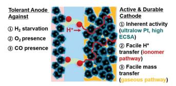
Fig. 1 Illustrative description that fuel cell catalysts should satisfy for MEA operation.
