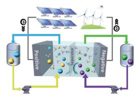
Fig. 1 A schematic diagram of a VFB
