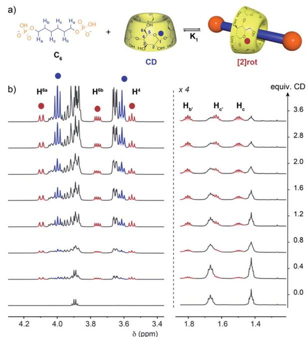
Fig. 2 (a) Equilibrium of formation of [2]pseudorotaxane between  $\alpha$ -CD and the  $C_6$  axle. (b)  $^1H$  NMR (600 MHz,  $D_2O$ , 300 K) titration of the  $C_6$  axle (2.8 mM) with CD in acetate buffer at pH = 5 showing the progressive appearance of [2]rot (red) and free CD (blue).
