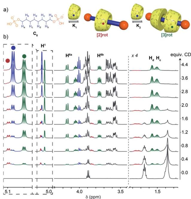
**Fig. 3** (a) Equilibrium of formation of [2] and [3]pseudorotaxanes with the C<sub>8</sub> axle. (b) <sup>1</sup>H NMR (600 MHz, D<sub>2</sub>O, 300 K) titration of the C<sub>8</sub> axle (2.8 mM) with CD in acetate buffer at pH = 5 showing the progressive appearance of [2]rot (red), [3]rot (green) and free CD (blue).
