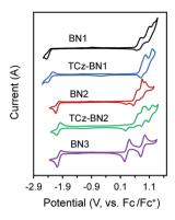
Fig. 4 Cyclic voltammograms (CV) for all compounds. The CV curves were measured at room temperature with 0.1 M solution of  $[n-Bu_4N]$  PF<sub>6</sub> in dichloromethane for the oxidation and reduction scan (vs. Fc/Fc<sup>+</sup>).
