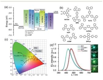
Fig. 6 (a) Device structures and energy level diagrams of devices i and ii. (b) Molecular structures of the functional materials used in OLED devices. (c) The CIE 1931 chromaticity diagram and (d) EL spectra of devices recorded at 1000 cd m<sup>-2</sup>. Photographs showing the emission colours of the device at a luminance  $\approx 1000$  cd m<sup>-2</sup>.
