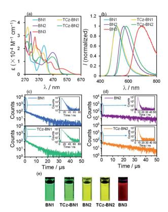
Fig. 5 (a) UV-Vis absorption spectra and (b) emission spectra (excitation at 406 nm, 398 nm, 465 nm, 464 nm and 531 nm for BN1, TCz-BN1, BN2, TCz-BN2 and BN3, respectively) of all five compounds; (c and d) transient PL decay curves in THF solution under  $\rm N_2$  conditions at 298 K; (e) photographs showing the emission colours of all five compounds.
