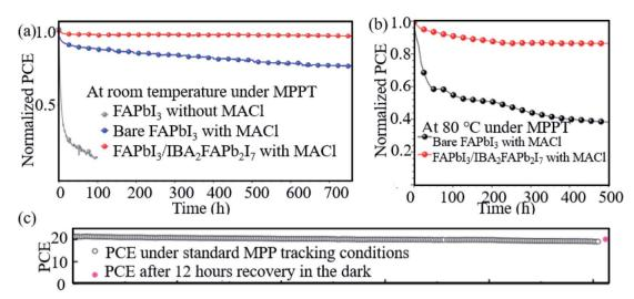
Fig. 9 Aging results (a) and (b) of PSCs based on bare FAPbl<sub>3</sub> (black dotted line) and  $\alpha$ -FAPbl<sub>3</sub>/IBA<sub>2</sub>FAPb<sub>2</sub>l<sub>7</sub> perovskites (red dotted line). Reprinted with permission from ref. 70, copyright 2020, Wiley. (c) Operational stability test of the vapor-treated FAPbl<sub>3</sub>-based PSCs under 500 hours of MPP-tracking conditions. Reprinted with permission from ref. 80, copyright 2020, Science Publishing Group.
