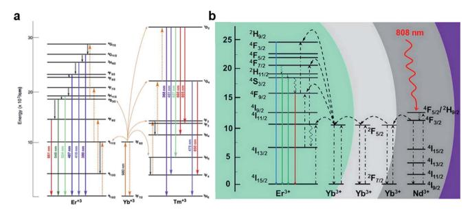
Fig. 1 Proposed energy transfer mechanism showing the UCL processes in (a)  $Er^{3+}$ ,  $Tm^{3+}$ , and  $Yb^{3+}$  doped UCNPs under 980 nm laser excitation<sup>31</sup> and (b)  $Nd^{3+}$ ,  $Yb^{3+}$ , and  $Er^{3+}$  doped UCNPs under 808 nm laser excitation.<sup>32</sup> Adapted from ref. 31 with permission from Elsevier Ltd, copyright 2014; adapted from ref. 32 with permission from American Chemical Society, copyright 2016.
