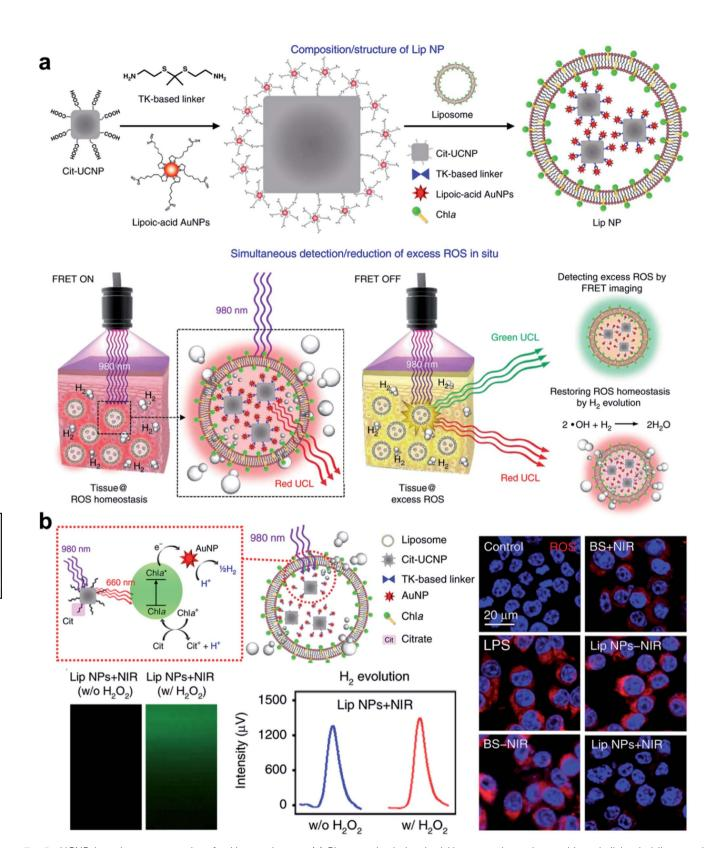
Fig. 5 UCNP-based nanocomposites for  $H_2$  gas therapy. (a) Photosynthesis-inspired  $H_2$  generation using a chlorophyll-loaded liposomal UCNP-based nanoplatform to (b) detect and scavenge excess ROS.<sup>42</sup> Adapted from ref. 42 with permission from Nature Publishing Group, copyright 2020.
