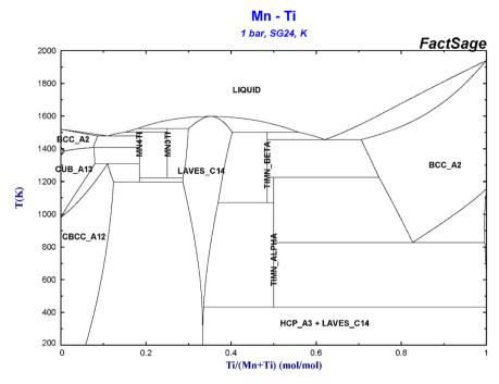
Fig. 2 Binary phase diagram of Mn-Ti.57,58
