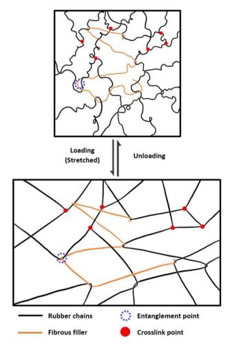
Fig. 7 Mechanical strength reinforcement by fibrous fillers through physical entanglement.117
