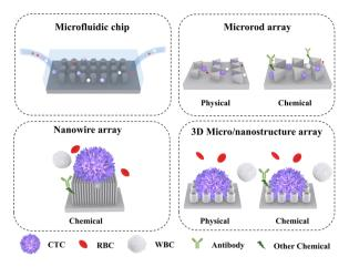
Fig. 1 Schematic illustrations of (A) micro-/nanostructure integrated microfluidic device for CTC capture. (B) 1D microrod arrays. (C) 1D nanowire array. (D) 3D hierarchical micro-/nanostructure arrays.
