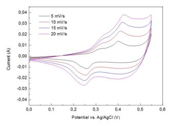
Fig. 20 CVA curves for nickel foam electrode with Ni-doped CuO nanolayers at a scan rate of 5, 10, 15 and 20 mV s $^{-1}$ .135
