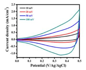
Fig. 25 Cyclic voltagramms of CuO with various scan rates of 1 M KOH electrolyte.  $^{149}$
