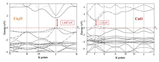
Band structures of Cu<sub>2</sub>O and CuO unit cells are drawn by CASTEP using LDA + U.
