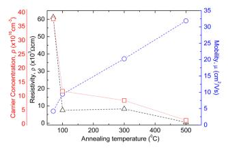
Fig. 16 Representation of the change of resistivity, mobility, and carrier concentration of copper oxide ( $Cu_2O$  and CuO) films with annealing temperature.<sup>123</sup>
