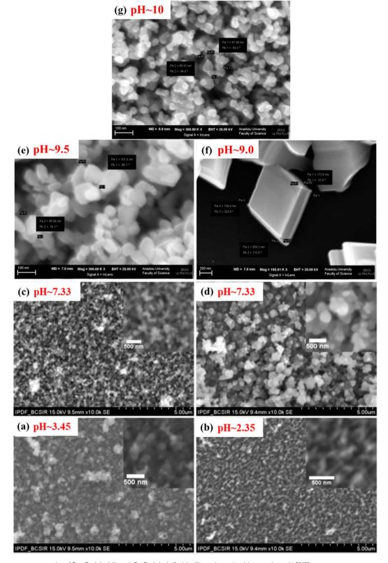
Fig. 6 SEM images representing {Cu $_2$ O: (a)–(d) and CuO: (e)–(g)} thin films deposited by varying pH. <sup>36,105</sup>
