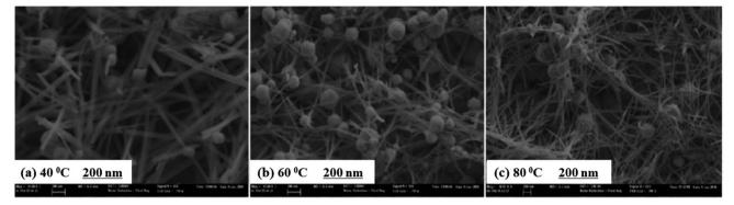
Fig. 13 SEM images of Cu<sub>2</sub>O nanostructured thin films deposited by SILAR at different bath temperatures (a) 40 °C, (b) 60 °C, and (c) 80 °C, <sup>112</sup>
