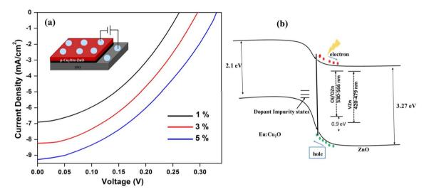
Fig. 18 (a) 1%, 3% and 5% Eu doped thin films having current-voltage characteristics of ITO/ZnO NRs/Eu: Cu<sub>2</sub>O/Al cell, (b) carrier transport and band structure of p-n junction.129
