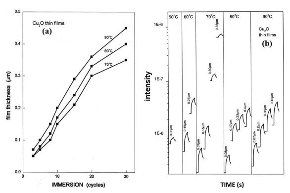
Fig. 12 Samples in NaOH solution (a) at different temperatures as a function of film thickness and immersions. (b) At the designated temperatures to record the photocurrent response of the  $Cu_2O$  thin films of different thicknesses.<sup>111</sup> [Light source: tungsten-halogen, intensity of illumination: 1 kW m<sup>-2</sup>, time length: 60–180 s, bias: 1 V applied across Ag print electrodes 5 mm (long)  $\times$  5 mm (separation)].
