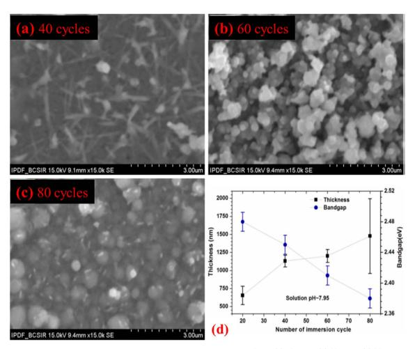
Fig. 9 SEM micrographs of the films grown with different immersion cycles at pH: 7.95 for (a) 40 cycles (b) 60 cycles (c) 80 cycles and (d) film thickness of  $Cu_2O$  thin films using different immersion cycles grown by m-SILAR.<sup>37</sup>
