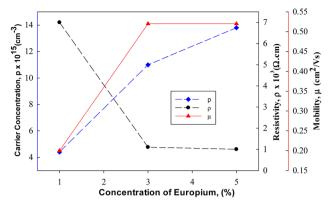
Fig. 17 Resistivity, carrier concentration and mobility for Eu doped Cu<sub>2</sub>O films.<sup>129</sup>
