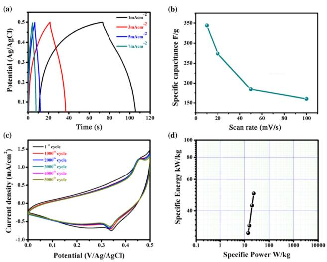
Fig. 26 (a) Representation of galvanostatic charge-discharge curves of CuO at diverse current densities. (b) Change of specific capacitance with scan rate (c) study of stability of CuO thin films (d) specific energy versus specific power of Ragone plot.<sup>149</sup>
