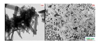
Fig. 22 (a) TEM (b) SEM images of the  $\rm Cu_2O$  grains showing needle-shaped uniformity on the surface. <sup>146</sup>
