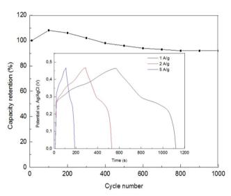
Fig. 21 The cycling stability for the Ni Foam electrode with Ni-doped CuO nanolayers at 2 A  $\rm g^{-1}$  whereas the inset graph represents galvanostatic charge–discharge curves of the electrode with Ni-doped CuO nanolayers. <sup>135</sup>
