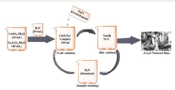
Fig. 3 Synthesis of the copper(1) oxide nanorod thin films. 93
