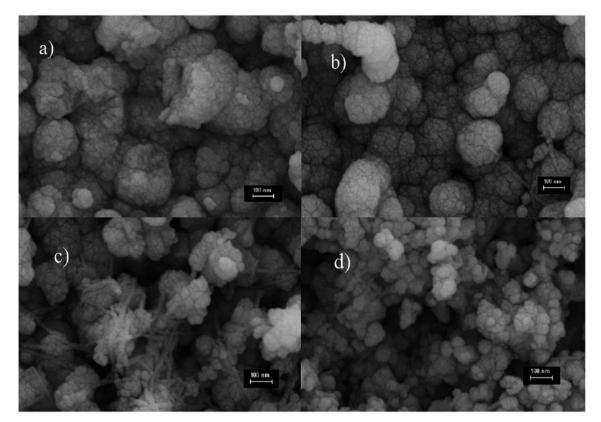
Fig. 5 The FE-SEM images of Cu<sub>2</sub>O nanostructured thin films deposited from four different Cu salts<sup>96</sup> (a) (CH<sub>3</sub>COO)<sub>2</sub>Cu·H<sub>2</sub>O, (b) CuSO<sub>4</sub>·5H<sub>2</sub>O, (c)  $Cu(NO_3)_2 \cdot 3H_2O$ , and (d)  $CuCl_2 \cdot 2H_2O$ .
