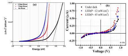
Fig. 7 (a) Variation of band gap with rinsing steps. (b) I-V characteristic curve for FTO/Cu<sub>2</sub>O/ZnO heterojunction cell grown on FTO substrate at pH-7.95. $^{101}$
