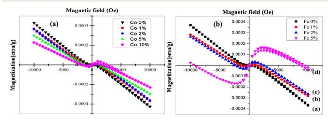
Fig. 19 Magnetic behavior of (a) Co-doped<sup>127</sup> (b) Fe-doped Cu<sub>2</sub>O thin films.<sup>128</sup>
