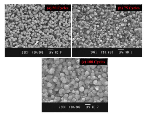
Fig. 10 SEM image of the Cu<sub>2</sub>O nanostructured films deposited at (a) 50 (b) 75 and (c) 100 dipping cycles. 105
