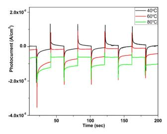
Fig. 23 PEC measurement of  $\text{Cu}_2\text{O}$  thin films at different bath temperatures.<sup>111</sup>
