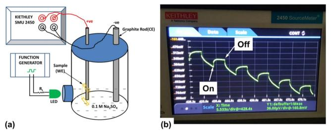
Fig. 27 (a) A representation of the transient surface photovoltage measurement system; (b) measurement of a typical Cu<sub>2</sub>O/FTO electrode in a PEC with  $0.1 \text{ M Na}_2\text{SO}_4$  electrolyte followed by real-time measurement in SMU 2450 demonstrating the shape of the LED modulated transient surface photovoltage.36
