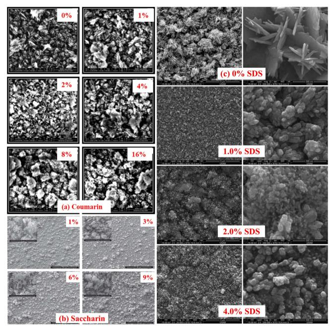
Fig. 14 SEM images of CuO nanostructured thin films as a function of different additive concentrations, such as (a) coumarin, 115 (b) saccharin and (c) SDS. 117
