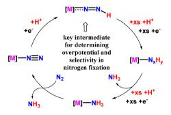
Fig. 35 Transition metal mediated catalytic N<sub>2</sub>RR mechanism for ammonia synthesis
