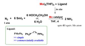
Fig. 23 Ammonia production at ambient reaction conditions by molybdenum complexes formed in situ by reacting [Mol $_3$ (THF) $_3$ ] and monodentate and bidentate phosphines.
