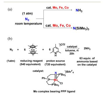
Fig. 10 (a) Ammonia or silylamine formation from dinitrogen using Mo, Fe, and Co catalyst at ambient reaction condition. (b) Catalytic nitrogen fixation using a molybdenum catalyst bearing PPP ligand.
