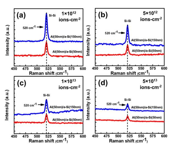
Fig. 7 Raman spectra of set-A and set-B samples irradiated at 100 °C with different fluences of (a)  $1 \times 10^{12}$  ions per cm<sup>2</sup>, (b)  $5 \times 10^{12}$  ions per  $\text{cm}^2$ , (c)  $1 \times 10^{13}$  ions per  $\text{cm}^2$ , and (d)  $5 \times 10^{13}$  ions per  $\text{cm}^2$ . (All figures are plotted in same y-scale range for comparison). [Reproduced/adapted from Maity et al., 157 RSC Adv., 2020, 10, 4414, with permission from The Royal Society of Chemistry.]
