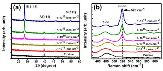
Fig. 10 (a) XRD pattern (b) Raman spectra of pristine sample and the samples irradiated with different ion fluence of  $7 \times 10^{14}$  ions per cm<sup>2</sup>,  $1 \times 10^{15}$  ions per cm<sup>2</sup>,  $3 \times 10^{15}$  ions per cm<sup>2</sup>,  $7 \times 10^{15}$ , and  $1 \times 10^{16}$  ions per cm<sup>2</sup>. [Reproduced/adapted from Maity *et al.*, <sup>161</sup> *J. Appl. Phys.*, 2022, **132**, 095303, with the permission from AIP Publishing.]
