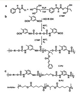
Fig. 9 Synthesis of photocrosslinkable polyurethane containing cinnamoyl. This figure has been adapted from ref. <sup>53</sup> with permission from Royal Society of Chemistry, copyright 2019.
