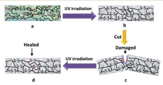
Fig. 2 Schematic of preparation and self-healing behavior of UV-curable material based on disulfide bond exchange: (a) before UV irradiation; (b) after UV irradiation; (c) damaged material; (d) self-healed material This figure has been adapted from ref. 24 with permission from Elsevier, copyright 2019.
