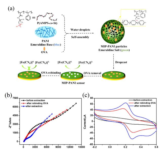
Fig. 3 (a) Schematic illustration of the synthesis of MIP-PANI particles and the fabrication of MIP-PANI sensor, (b) EIS curves and (c) CV curves of MIP-PANI particles modified electrode in  $[Fe(CN)6]^{3-/4-}$  solution before extraction, after extraction and after rebinding OVA by incubation in 0.5 mg mL<sup>-1</sup> OVA solution (reprinted with permission from Elsevier, ref. 21 Luo *et al.*, (2017)).
