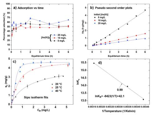
Fig. 7 (a) Adsorption vs. time; (b) pseudo 2nd order model; plots of initial As(III) concentrations of 5, 10, and 20 mg L<sup>-1</sup>; (c) the Sips isotherm fits of As(III) adsorption; and (d) van't Hoff plot of  $\ln K_s vs. 1/T$  for the As(III) adsorption. Reproduced from ref. 95 with permission from Elsevier, copyright
