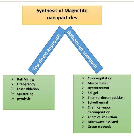
Fig. 4 Techniques to synthesize magnetite nanoparticles.
