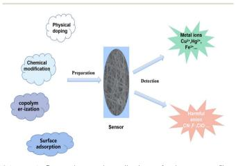
**Scheme 1** Preparation and application of electrospun fiber membrane ion sensor.
