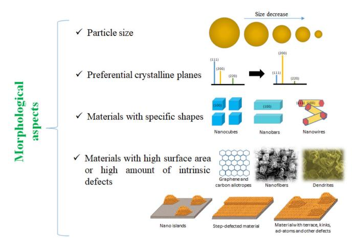
Morphological aspects of nanomaterials which can be modified/tuned to enhance the creatinine electrochemical detection.
