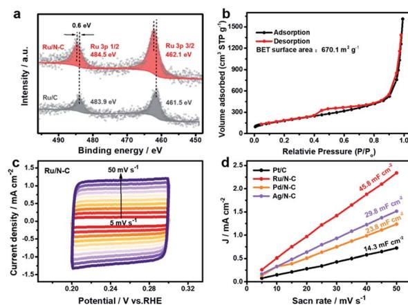
Fig. 5 (a) High-resolution XPS spectra of Ru 3p; (b)  $N_2$  adsorption-desorption isotherm of Ru/N-C; (c) cyclic voltammetry curves of Ru/N-C at various scan rates from  $5$ – $50 \text{ mV s}^{-1}$  in the region of  $0.20$ – $0.28 \text{ V}$  vs. RHE; (d)  $C_{dl}$  comparison of Ru/N-C, commercial Pt/C, Pd/N-C and Ag/N-C.
