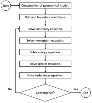
Fig. 4 Model solving algorithm.
