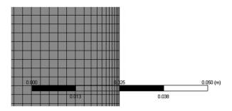
Fig. 3 Inflation method close up view.
