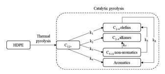
Fig. 2 Kinetic scheme for the reaction. Adapted from Artetxe et al.8
