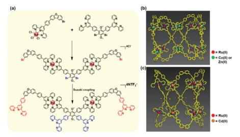
Fig. 1 (a) Synthesis of ligand L, (b) representative energy-minimized structure of Co<sub>8</sub>L<sub>4</sub> (Zn<sub>8</sub>L<sub>4</sub>), and (c) representative energy-minimized structure of Cd<sub>6</sub>L<sub>3</sub>.
