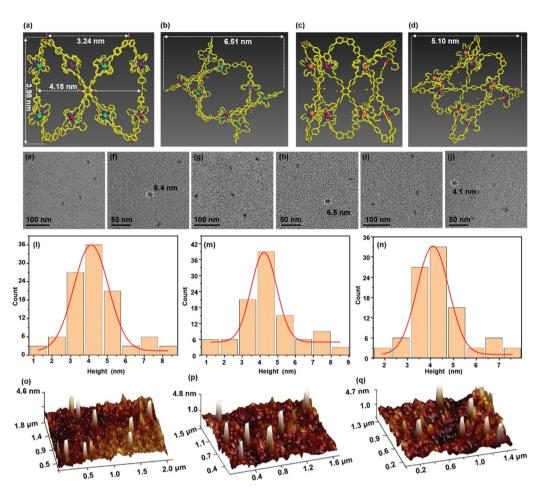
Fig. 4 (a) and (b) Representative energy-minimized structure of  $Co_8L_4$  ( $Zn_8L_4$ ), (c) and (d) representative energy-minimized structure of  $Cd_6L_5$ , (e) and (f) TEM images of Co<sub>8</sub>L<sub>4</sub>, (g) and (h) TEM images of Zn<sub>8</sub>L<sub>4</sub>, (i) and (j) TEM images of Cd<sub>6</sub>L<sub>3</sub>, (l)-(n) AFM height statistical histogram for 100 particles of  $Co_8L_4$ ,  $Zn_8L_4$ , and  $Cd_6L_3$ , and (o)-(q) AFM images of  $Co_8L_4$ ,  $Zn_8L_4$  and  $Cd_6L_3$ .
