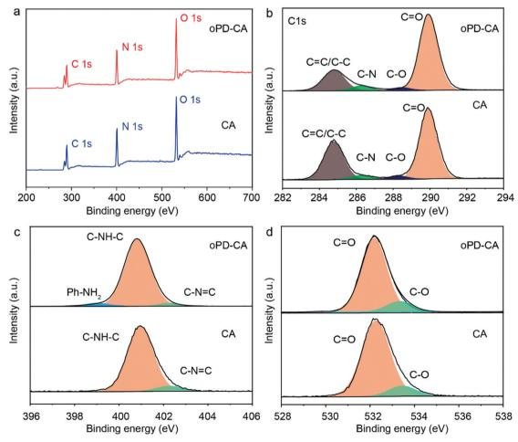
Fig. 2 XPS spectra of oPD-CA and CA for (a) survey scan, (b) C1s, (c) N1s, and (d) O1s.
