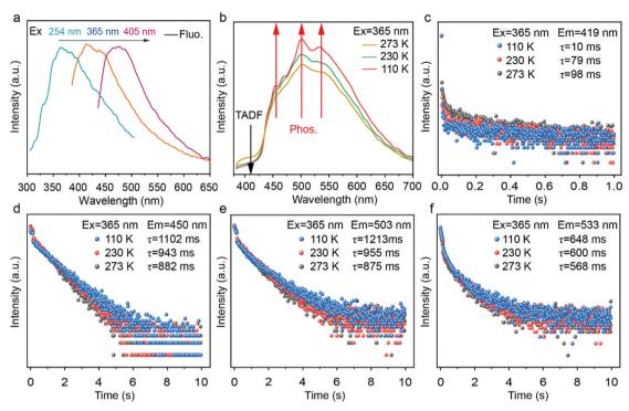
Fig. 3 (a) Excitation wavelength dependent room-temperature fluorescence spectra, (b) temperature-dependent afterglow spectra, (c) TADF decay kinetics, (d) phosphorescence decay kinetics for 503 nm, and (f) phosphorescence decay kinetics for 533 nm.
