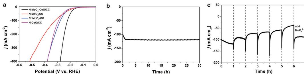
**Fig. 2** (a) LSV curves of NiMoO<sub>4</sub>-CoO/CC, NiMoO<sub>4</sub>/CC, CoMoO<sub>4</sub>/CC, and NiCoO/CC. (b)  $J-t$  curve of NiMoO<sub>4</sub>-CoO/CC in 1.0 M KOH. (c)  $J-t$  curve of NiMoO<sub>4</sub>-CoO/CC obtained by renewing the electrolyte every 1 hour.
