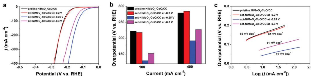
**Fig. 3** (a) LSV curves, (b) overpotentials at current densities of 100 and 400 mA cm<sup>-2</sup>, and (c) Tafel plots of pristine NiMoO<sub>4</sub>-CoO/CC, act-NiMoO<sub>4</sub>-CoO/CC at -0.2 V, act-NiMoO<sub>4</sub>-CoO/CC at -0.25 V, and act-NiMoO<sub>4</sub>-CoO/CC at -0.3 V.
