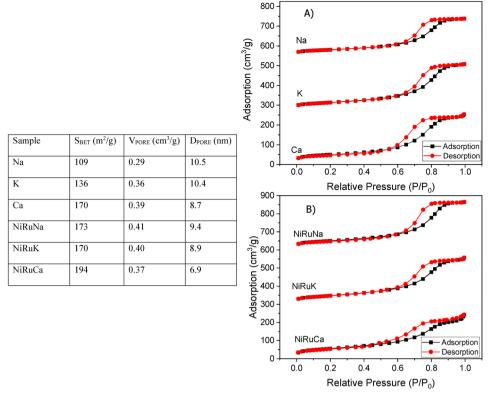
Fig. 8 Textural properties of the materials on the left-hand side and nitrogen adsorption-desorption isotherms of the (A) supported adsorbents and (B) DFMs on the right-had side.
