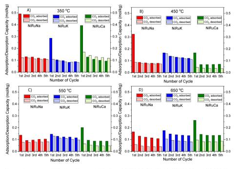
Fig. 2 CO<sub>2</sub> Adsorption/desorption cycles of NiRuNa, NiRuK and NiRuCa at (A) 350 °C, (B) 450 °C, (C) 550 °C and (D) 650 °C.
