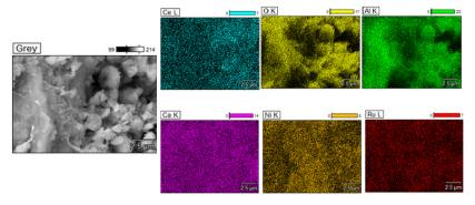
Fig. 13 SEM and EDX mapping of NiRuCa.
