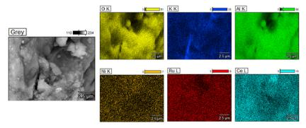
Fig. 12 SEM and EDX mapping of NiRuk.
