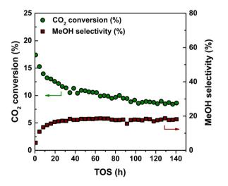
Fig. 1 CO<sub>2</sub> conversion and methanol selectivity as a function of time on stream (TOS) for the 4.7\_Cu/C catalyst with 5.2 wt% Cu. Reaction conditions: 4.2 mg of Cu per reactor, 40 bar(g), 260 °C, 600 mL min<sup>-1</sup>  $g_{Cu}^{-1}$ ,  $H_2/CO_2/He = 67.5/22.5/10$  vol%.
