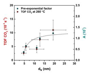
Fig. 4 TOF and pre-exponential factor as a function of Cu particle size. Line is drawn to guide the eye. Reaction conditions: 4.2 mg of Cu per reactor, 40 bar(g), 260 °C, 600 mL min<sup>-1</sup>  $g_{Cu}^{-1}$ ,  $H_2/CO_2/He = 67.5/22.5/$
