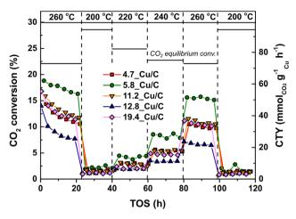
Fig. 3 Characteristic profiles for CO<sub>2</sub> conversion and weight-normalized copper time yield for Cu/C catalysts as function of TOS (h) at different temperatures. Reaction conditions: 4.2 mg of Cu per reactor, 40 bar(g), 600 mL min<sup>-1</sup>  $g_{Cu}^{-1}$ ,  $H_2/CO_2/He = 67.5/22.5/10 vol%.$
