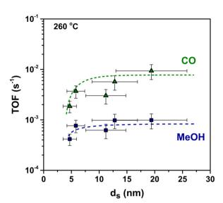
Fig. 6 MeOH and CO TOF as a function of the Cu particle size. Trend lines were added to guide the eye. Reaction conditions: 4.2 mg of Cu per reactor, 40 bar(g), 260 °C, 600 mL min<sup>-1</sup>  $g_{Cu}^{-1}$ ,  $H_2/CO_2/He = 67.5/22.5/10$  vol%.
