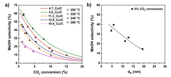
Fig. 5 (a) MeOH selectivity as a function of  $CO_2$  conversion for catalysts with different Cu particle sizes. (b) Selectivity to MeOH as a function of Cu particle size for a  $CO_2$  conversion of  $\sim$ 5%. The trend line was added to guide the eye. Reaction conditions: 4.2 mg of Cu per reactor, 40 bar(g), 600 mL min<sup>-1</sup>  $g_{Cu}^{-1}$ ,  $H_2/CO_2/He = 67.5/22.5/10$  vol%.
