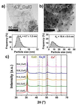
Fig. 2 Transmission electron micrographs with corresponding particle size distributions of the 4.7\_Cu/C (a) and 19.4\_Cu/C (b) catalysts after activation. (c) Powder X-ray diffractograms of the activated Cu/C catalysts, diffractograms normalized to the intensity of the carbon (002) diffraction peak and vertically offset for clarity.
