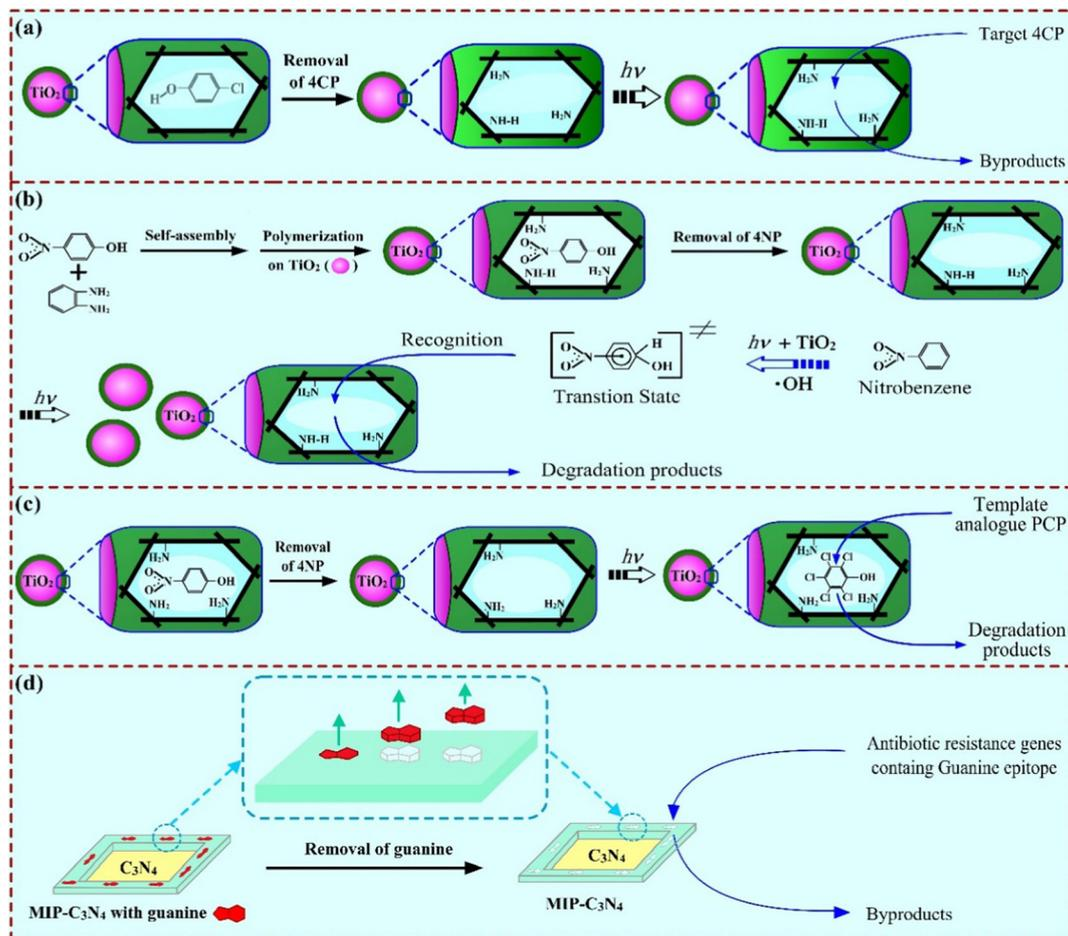
Fig. 7 Schematic route for preparation of (a) RS-MIPCs *via* surface imprinting, adapted with permission from ref. 17; (b) TSA-MIPCs, adapted with permission from ref. 80; (c) SA-MIPCs, adapted with permission from ref. 77, and (d) RS-MIPCs by using an epitope imprinting method, adapted with permission from ref. 81.
