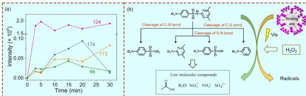
Fig. 10 (a) UPLC-MS intensity changes of the intermediate products at different reaction times during the photodegradation of SM2 over imprinted MIL-101-NH<sub>2</sub>. (b) Proposed SM2 degradation pathways over the imprinted MIL-101-NH<sub>2</sub>. Adapted with permission from ref. 98.
