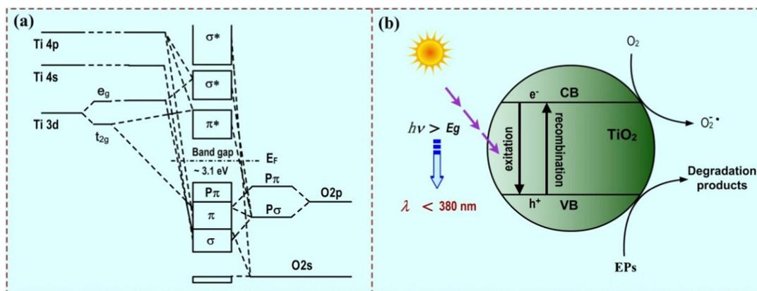
Fig. 2 (a) Schematic representation of molecular orbital interactions between titanium (Ti) and oxygen (O) of  $TiO_2$  semiconductors. Adapted with permission from ref. 27. (b) Schematic representation of the photodegradation of EPs on  $TiO_2$  semiconductors.
