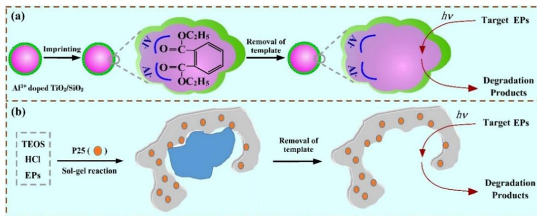
Fig. 3 (a) Schematic route for preparation of inorganic MIP-coated photocatalysts. Adapted with permission from ref. 34. (b) Schematic route for synthesis of MIPCs *via* an acid-catalyzed sol-gel route. Adapted with permission from ref. 35.
