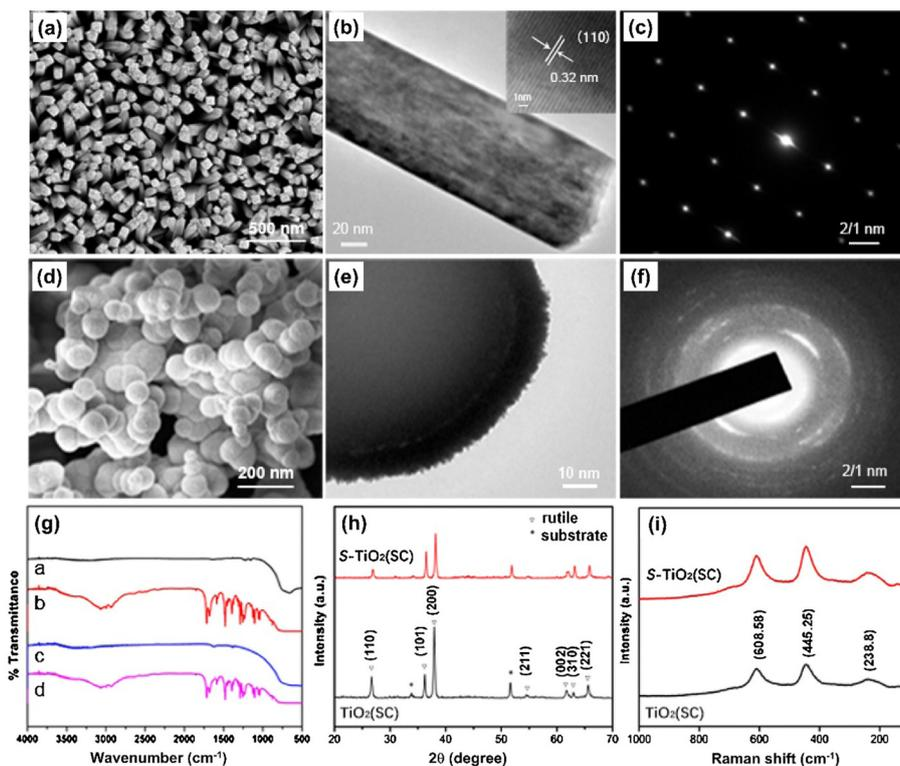
Fig. 11 (a), (d) FE-SEM images, (b), (e) TEM images, (insets: the corresponding HRTEM images), and (c), (f) SAED patterns of S-TiO<sub>2</sub> (HTS) and S-TiO<sub>2</sub> (LPD), respectively. (g) FTIR spectra of S-TiO<sub>2</sub>, (h) XRD and (i) Raman spectra of TiO<sub>2</sub> (SC) and S-TiO<sub>2</sub> (SC). Adapted with permission from ref. 75.
