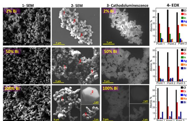
**Fig. 1** SEM microphotographs of CANBIC microcrystals made by using the secondary electrons contrast (columns 1 and 2) and the cathodoluminescence contrast (column 3) as well as elemental composition in selected points determined by EDX (column 4).
