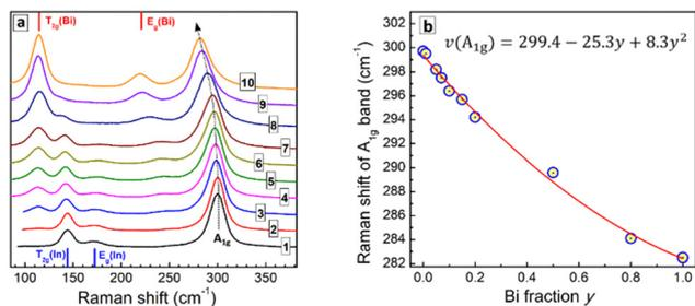
Fig. 6 (a) Raman spectra of CANBIC perovskites with varied Bi fraction  $y = 0$  (1), 0.01 (2), 0.05 (3), 0.07 (4), 0.10 (5), 0.15 (6), 0.20 (7), 0.50 (8), 0.80 (9), and 1.00 (10). (b) Frequency of the  $A_{1g}$  mode as a function of Bi fraction  $y$  (scatter). Solid red line represents the best fit with a polynomial function " $\nu(A_{1g})$  versus  $y$ " presented in the figure.
