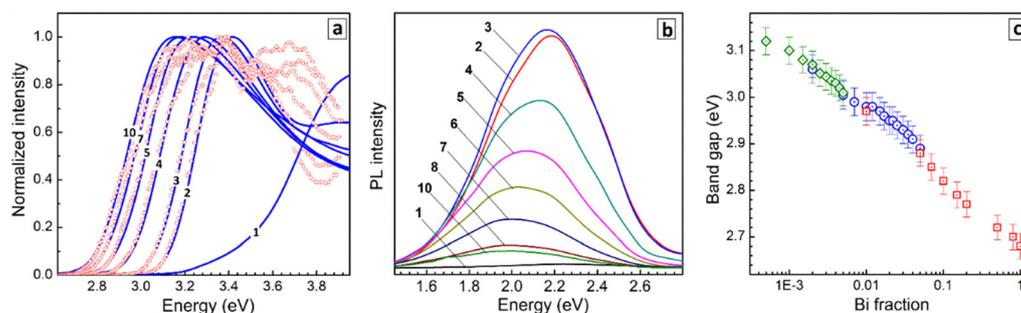
Fig. 3 (a and b) Absorption, PL excitation (a), and PL (b) spectra of CANBIC perovskites with Bi fraction  $y = 0$  (curve 1), 0.01 (2), 0.05 (3), 0.07 (4), 0.10 (5), 0.15 (6), 0.20 (7), 0.50 (8), 0.90 (9), and 1.00 (10). In (a) solid lines are absorption spectra and circles represent corresponding PL excitation spectra. (c) Band gap of CANBIC perovskites as a function of Bi fraction  $y$ . A legend for different symbols in (c) is provided in the caption of Fig. 4.
