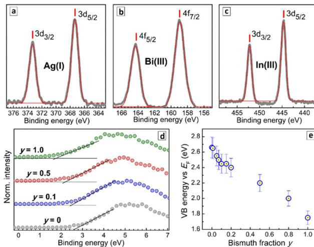
Fig. 5 (a–c) High-resolution X-ray photoelectron spectra of CANBIC perovskite with  $x = 0.4$  and  $y = 0.5$  in the range of Ag3d (a), Bi4f (b), and In3d (c) electron binding energies. Gray lines represent experimental spectra, red lines fits with Gaussian profiles. (d) X-Ray photoelectron spectra of CANBIC perovskites in the VB region. (e) VB energy with respect to the Fermi level  $E_F$  as a function of Bi fraction  $y$  in CANBIC perovskites.
