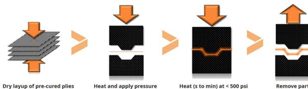
Fig. 19 Pre-cured vitrimer matrix composite in mould consolidation cycle.<sup>99</sup>
