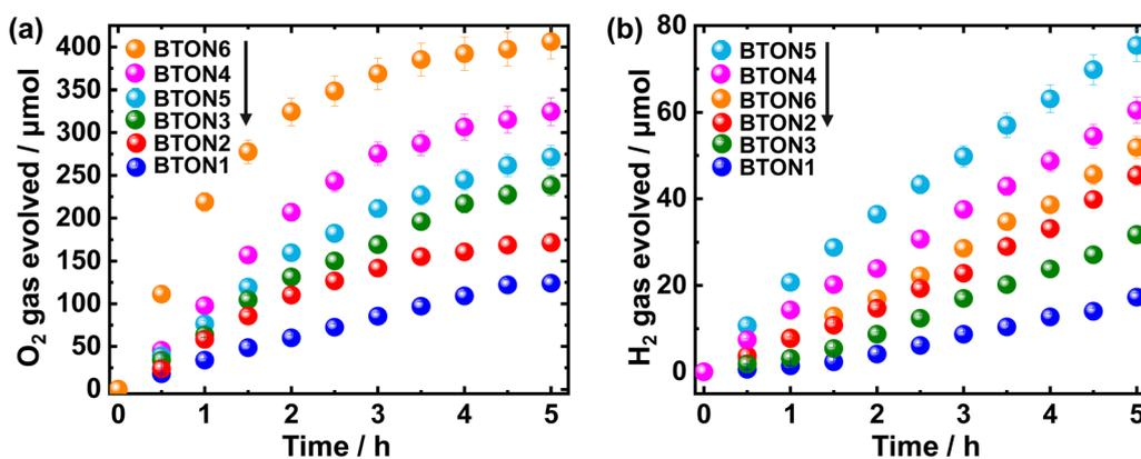
Fig. 6 Reaction time courses for photocatalytic O<sub>2</sub> (a) and H<sub>2</sub> (b) evolution over BTON1, BTON2, BTON3, BTON4, BTON5, and BTON6 loaded with CoO<sub>x</sub> and Pt nanoparticles as O<sub>2</sub> and H<sub>2</sub> evolution cocatalysts under visible light irradiation.
