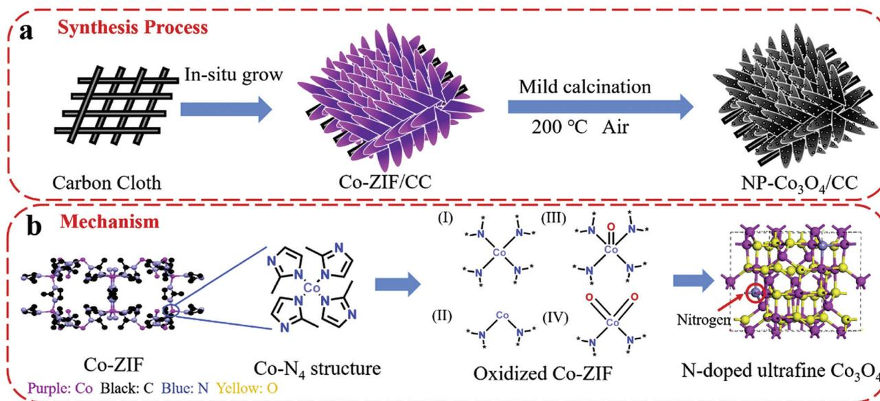
Fig. 14 Schematic demonstration of (a) the fabrication process of NP- $\text{Co}_3\text{O}_4/\text{CC}$  and (b) the proposed mechanism of nitrogen doping in cobalt oxide lattices. Reproduced from ref. 282 with permission from Elsevier B.V.
