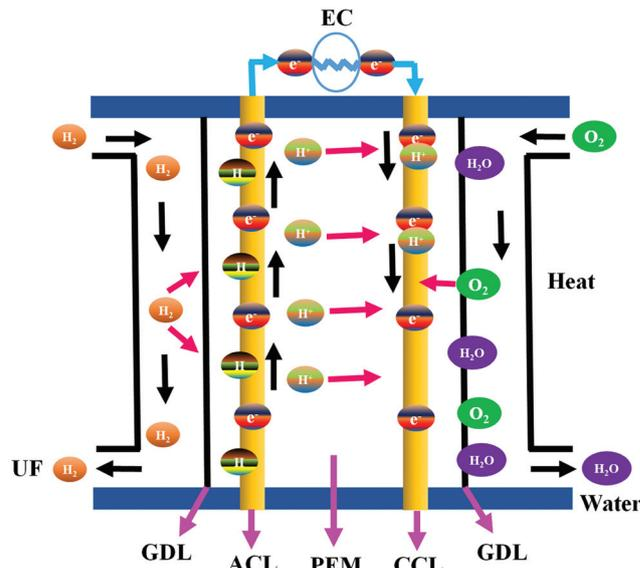
Fig. 3 The working principle of PEMFCs (note: H<sub>2</sub> – hydrogen, O<sub>2</sub> – oxygen, H<sub>2</sub>O – water, UF – unused fuel, GDL – gas diffusion layer, ACL – anode catalyst layer, PEM – proton exchange membrane, CCL – cathode catalyst layer, H<sup>+</sup> – proton, e<sup>-</sup> – electron).
