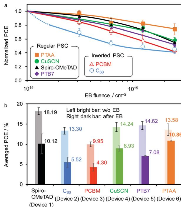
Fig. 5 (a) Normalized PCE of various PSCs upon EB exposure. (b) Average PCE values with error bars (standard deviation) before (left bar) and after EB (right bar,  $F_{\text{EB}} = 2.5 \times 10^{15} \text{ cm}^{-2}$ ) exposure.
