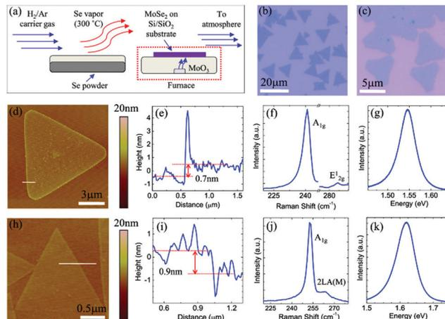
**Fig. 5** (a) Schematic of the AP-CVD setup used for the growth of 2D TMDCs such as MoSe<sub>2</sub>. Optical microscopy images of (b) MoSe<sub>2</sub> and (c) WSe<sub>2</sub> monolayer domains grown on Si/SiO<sub>2</sub>. AFM image, height profile across the line marked on the AFM image, and Raman and PL spectra of (d–g) MoSe<sub>2</sub> and (h–k) WSe<sub>2</sub>. (Figure reproduced from ref. 92.)
