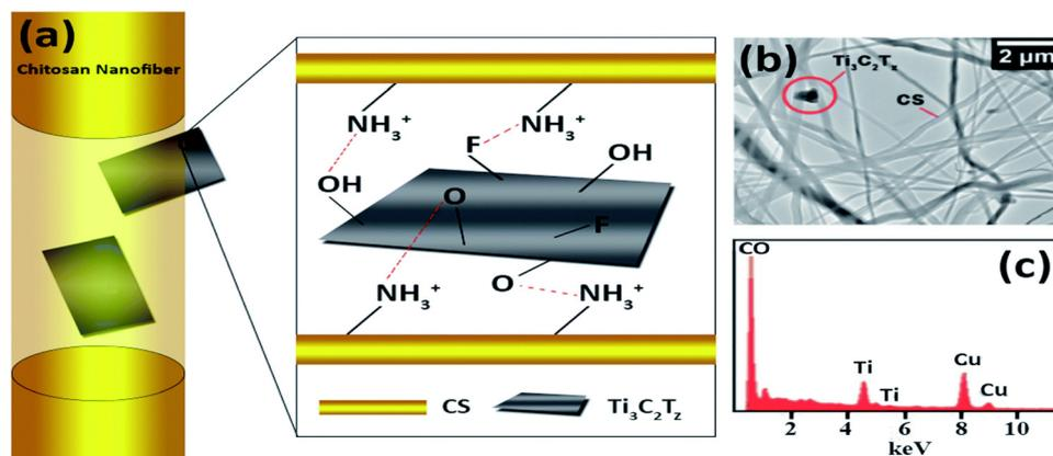
Fig. 8 (a) Schematic representations of the observed orientations of  $Ti_3C_2T_z$  flakes inside chitosan nanofibers. (b) Transmission electron microscopy image of the  $Ti_3C_2T_z$ /CS nano-fibers and (c) elemental examination (presence of copper is attributed to the TEM grid). (Adapted from ref. 143 under Creative Commons License 3.0, Copyright©2018, The Royal Society of Chemistry.)
