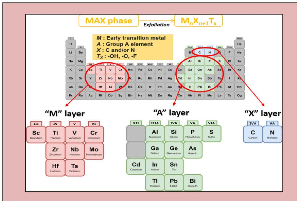
Fig. 1 Composition of the general elements of MXenes and MAX phases, where M is an early transition metal, A is a group A element, X is N and/or C, and T<sub>x</sub> is a surface functional group (adapted from ref. 46 under Creative Commons Attribution 4.0).
