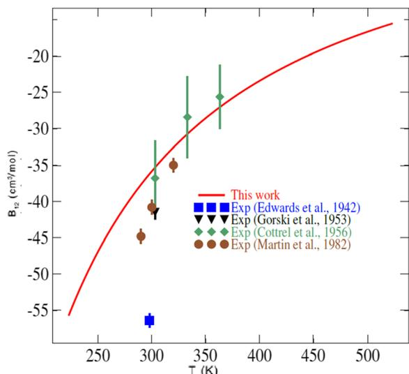
Fig. 7 Temperature dependence of the second virial coefficient of the CO<sub>2</sub>-O<sub>2</sub> mixture. The symbols are experimental values (Exp.) found in the literature.<sup>68–71</sup>
