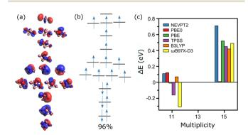
Fig. 6 (a) Plot of the active orbitals in the CASSCF calculation of Co<sub>5</sub><sup>+</sup>, ordered in ascending order of energy. (b) Diagram (not to scale) of the electronic levels of Co5+, with a representation of the electron occupancies in the M = 13 ground-state. (c) Energy differences, with respect to the measured multiplicity state (M = 13), for calculations conducted at the NEVPT2, DFT(PBE0), DFT(PBE), DFT(TPSS), DFT(B3LYP) and DFT(ωB97X-D3) levels of theory.
