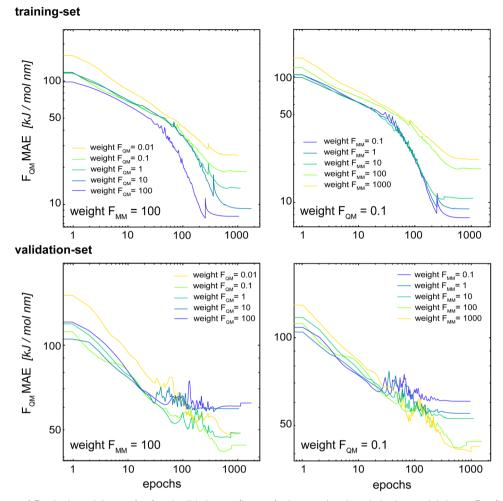
Fig. 6 Learning curves of  $F_{\text{OM}}$  in the training set (top) and validation set (bottom) when varying the relative loss weightings  $wF_{\text{OM}}$  (left) and  $wF_{\text{MM}}$  (right). The basic GCNN with the  $\Delta$ -learning scheme and the test system uracil in water was used. The weight of the energy loss (wE) is kept constant at 1.0.
