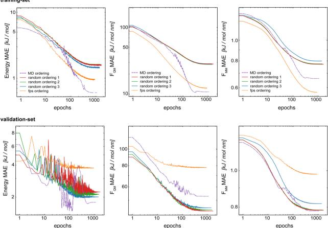
Fig. 8 Learning curves for the training set (top) and validation set (bottom) when varying the order of the data points in the training set. The Δ-learning GCNN for uracil in water is shown.
