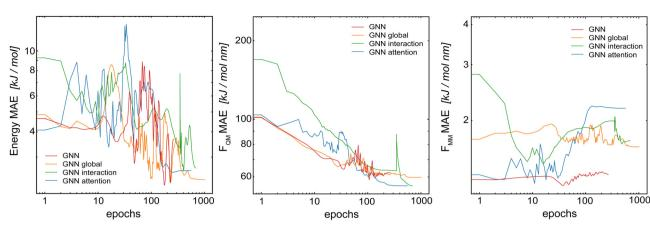
Fig. 3 Mean absolute error (MAE) on the validation set as a function of the training epochs (learning curves) of the  $\Delta$ -learning GCNN models containing global information for the test system uracil in water. (left): MAE of the energies in the QM zone. (middle): MAE of the forces on the QM particles. (right): MAE of the forces on the MM particles from the QM zone.
