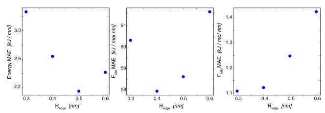
Fig. 4 Influence of  $R_{\text{edge}}$  on the mean absolute error (MAE) of the  $\Delta$ -learning basic GCNN model for uracil in water. (left): MAE of the energies in the QM zone. (middle): MAE of the forces on the QM particles. (right): MAE of the forces on the MM particles from the QM zone. The numerical values are given in Table 2.
