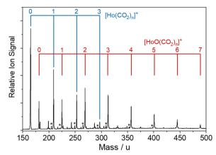
Fig. 2 Representative time-of-flight mass spectrum obtained following the laser ablation of a Ho target in the presence of a backing gas mixture of ca. 2.5%  $CO_2$  in Ar.  $Ho(CO_2)_0^+$  and  $[HoO(CO_2)_0]^+$  complexes are formed in high number density, together with Ar-tagged species (marked with asterisks). Other, unmarked peaks result from background H2O adsorption to the clusters.
