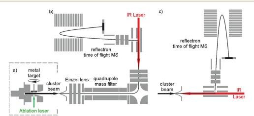
Fig. 1 Schematic of the instruments used for infrared action spectroscopy of  $[HoO_m(CO_2)_n]^+$  complexes. The cutaway source, (a), is common to both experiments. In variant (b) a quadrupole mass filter-bender assembly (Extrel) provides parent ion mass selection. In (c) IR-induced depletion of a wide range of Ar-tagged complexes is recorded simultaneously. In both cases infrared excitation occurs before detection.
