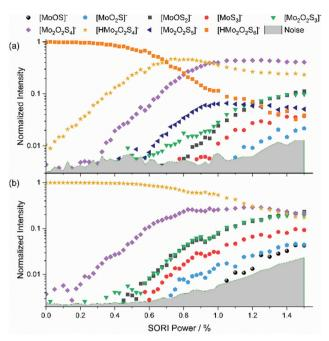
Fig. 3 (a) SORI-CID fragmentation curve of (a)  $[{\rm HMo_2O_2S_6}]^-$  and (b)  $[{\rm HMo_2O_2S_4}]^-.$
