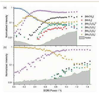
Fig. 1 Fragmentation curve obtained from the SORI-CID experiment of (a)  $[Mo_2O_2S_6]^{2-}$  and (b)  $[Mo_2O_2S_6]^{-}$ .
