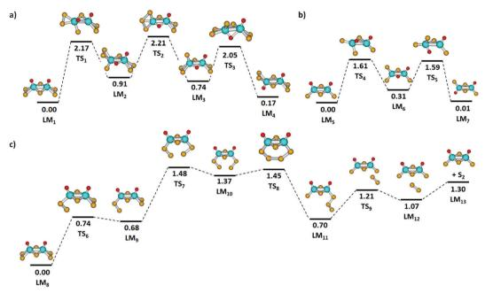
Fig. 5 Reaction pathways for isomerization reactions in (a)  $[Mo_2O_2S_6]^{2-}$  and (b)  $[Mo_2O_2S_4]^{-}$  clusters. (c) Simplified reaction profile from  $[Mo_2O_2S_6]^{-}$  to  $[Mo_2O_2S_4]^- + S_2$ . Calculated at the B3LYP+D3/def2TZVP level; relative energies are given in eV, local minima (LM) and transition states (TS) are denoted. Color code: Mo - cyan, S - yellow, O - red, H - white.
