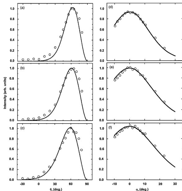
Fig. 7 In plane angular distributions (left panels) and out-of-plane angular distributions (right panels) for Ar scattering from molten Ga with an incident angle of  $55^\circ$  and incident energy of 0.95 eV for three different values of temperature: (a) and (d) 308 K, (b) and (e) 436 K, and (c) and (f) 586 K. Data from ref. 78 are open circles and calculations are the solid curves. (Reprinted with permission from ref. 79, Copyright [1997] American Institute of Physics.)
