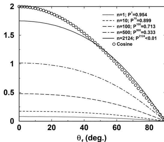
Fig. 12 The evolution of the final distribution in polar angle  $\theta_f$  for the same Ar/W system as in Fig. 11. The Knudsen cosine distribution is shown as open circles. (Reprinted with permission from ref. 94, Copyright [2008] American Physical Society.)
