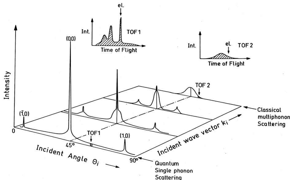
**Fig. 1** A depiction of the transition from quantum mechanical scattering (in the front) to classical scattering (in the rear) as a function of increasing incident particle wave vector (increasing energy). At low incident energies, sharp quantum features are observed in both the angular distributions and the energy-resolved TOF1 and TOF2 plots (insets), while at large energy only broad classical features appear. Courtesy of J. R. Manson and J. P. Toennies.
