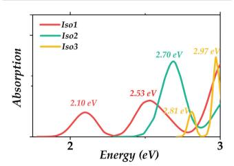
Fig. 5 Calculated optical absorption spectra for the three Au<sub>22</sub>(SR)<sub>16</sub>  $(R = CH_3)$  isomers.
