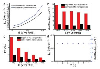
Fig. 2 (a) Total current densities for NH<sub>3</sub> production. (b) Yield rate and (c) faradaic efficiency for NH<sub>3</sub> production at different potentials over dispersed Ru nanoparticles and connected Ru nanoparticles. (d) The current density and yield rate for NH<sub>3</sub> production during a 7 h durability test at -0.1 V versus RHE over connected Ru nanoparticles.
