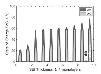
Fig. 7 Stability analysis of SEI growth, according to eqn (12). Filled areas show conditions of unstable SEI growth  $\tilde{s} > \partial \tilde{L}/\partial \tilde{t}$  depending on the SEI thickness h and the state of charge for increasing wavenumbers  $\tilde{k}$ .
