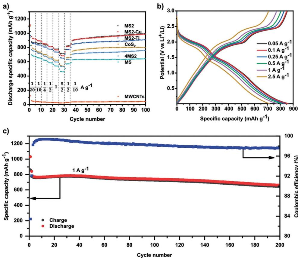
Fig. 6 (a) Galvanostatic rate performance test of all HESSs, CoS<sub>2</sub>, 4MS2, and MWCNTs half-cell at different current densities and 25 °C in the voltage range between 0.01 and 3 V versus Li<sup>+</sup>/Li. (b) Voltage profiles of MS2 half-cell at different currents. (c) Specific charge/discharge capacity of MS2 half-cell and Coulombic efficiency as a function of cycle number at 1 C and 25 °C in the range between 0.01 and 3 V. Copyright permission from Wiley, used from ref. 52.
