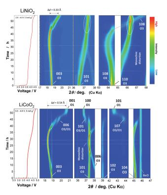
Fig. 2 Contour plots for selected ranges obtained from the in situ XRD patterns of LiNiO<sub>2</sub> and LiCoO<sub>2</sub> at a rate of 5 mA  $g^{-1}$ , and corresponding initial charge curves in electrochemical cells are also shown. The original in situ XRD data are shown in ESI Fig. S3.†
