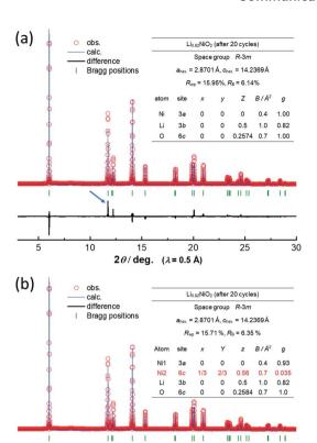
Fig. 4 Comparison of fitting results of Rietveld analysis of the synchrotron XRD pattern of  $\text{Li}_x\text{NiO}_2$  after the 20-cycle test (a) without and (b) with the presence of Ni ions at 6c tetrahedral sites. A clear deviation between simulated and observed patterns for the 101 diffraction line is noted in (a) as marked by the blue arrow.
