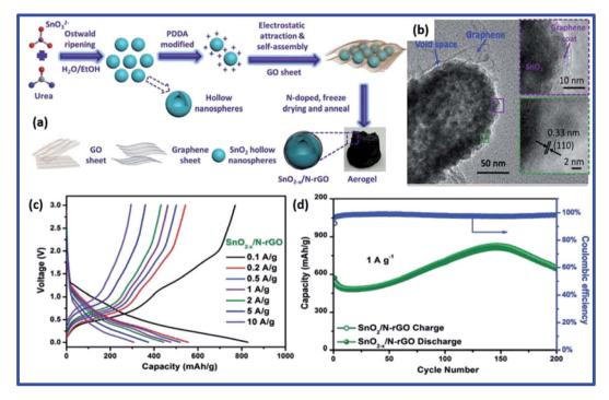
Fig. 29 (a) Scheme showing the preparation of a 3D hierarchical  $SnO_{2-x}/N$ -rGO network. (b) TEM images, with the insets showing the HRTEM images, (c) charge–discharge profiles, and (d) cycling performance (0.1 A g<sup>-1</sup>) of  $SnO_{2-x}/N$ -rGO, <sup>357</sup> presented with permission and copyright.
