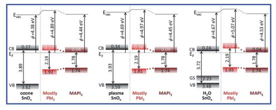
Fig. 21 Electronic structure of different SnO<sub>x</sub> variants in their pristine state and of a thin and thick (bulk-like) MAPbI<sub>3</sub> layer deposited on top of them. The energy level positions were determined by UPS and IPES measurements. Abbreviations— $E_{\text{vac}}$ : vacuum level; EF: Fermi energy; and  $\varphi$ : work function. The values written at the VB and the CB mark their distance from the Fermi energy, 302 presented with permission and copyright.
