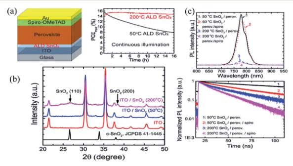
Fig. 24 (a) Schematic representation of plasma-assisted atomic layer deposition of the SnO<sub>2</sub> layer (glass/ITO/ALD SnO<sub>2</sub>/CH<sub>3</sub>NH<sub>3</sub>Pbl<sub>3</sub>/spiro-OMeTAD/Au) with its PCE performance; (b) XRD analysis of SnO2 at different annealing temperatures; and (c) steady state and time resolved photoluminescence of SnO<sub>2</sub>, presented with permission and copyright.<sup>301</sup>
