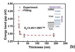
Fig. 2 (a) Impact of doping elements on conduction band offsets. (b) Thickness-dependent energy band gap of epitaxially grown Sb doped  $SnO_2$  using pulse laser deposition, presented with permission and copyright.<sup>74</sup>
