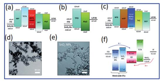
Fig. 12 Energy band diagrams of (a) red, (b) green, and (c) blue OLEDs with SnO2:Sb or ITO as the anode electrode. Reproduced with permission.97 Copyright: The Royal Society of Chemistry 2016. The TEM images of (d) ZnO or (e) SnO<sub>2</sub> NPs; (f) energy level diagram of QD-LEDs with ZnO or SnO<sub>2</sub> NPs as the ETLs. Reproduced with permission.<sup>213</sup> Copyright: The Royal Society of Chemistry 2020.
