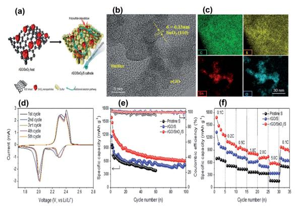
Fig. 32 Schematic representation of the rGO/SnO<sub>2</sub>/S cathode acting as a polysulphide immobilizer (a); HRTEM image (b) and elemental mapping (c) of the rGO/SnO<sub>2</sub>/S composite; cyclic voltammetry curve at  $0.1 \text{ mV s}^{-1}$  (d); and cycling performance (e) and rate performance (f) of the rGO/ SnO<sub>2</sub>/S composite.<sup>366</sup> Adapted with permission of Elsevier.
