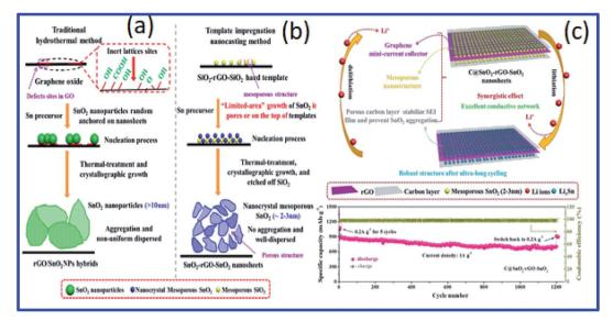
Fig. 28 Schematic representation of the research methodology adopted for the (a) hydrothermal method, (b) nanohard template casting method, and (c) charge/discharge profiles of  $C@SnO_2-rGO-SnO_2$  at a current density of 1 A  $g^{-1}$ , 356 presented with permission and copyright.
