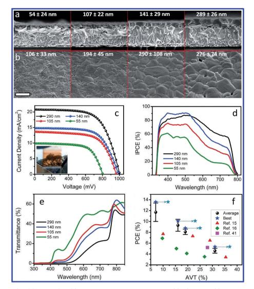
Fig. 25 (a) Cross-section SEM (b) top view SEM, (c) current density voltage characteristics, (d) IPCE spectra, (e) transmittance spectra and (f) PCE versus AVT plot for MAPbI<sub>3</sub> thin-film solar cells with different absorber layer thicknesses and a DMD cathode,  $^{311}$  presented with permission and copyright.
