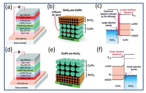
Fig. 13 Device structures of (a) normal OLEDs and (d) inverted OLEDs. (b and e) Schematic diagram and (c and f) energy band structure of the (b and c) diffused SnO<sub>2</sub>-on-CuPc and (e and f) abrupt CuPc-on-SnO<sub>2</sub> interface. Reproduced with permission.<sup>214</sup> Copyright: American Chemical Society 2011.
