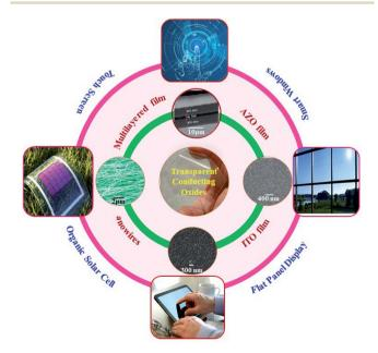
Fig. 1 Schematic diagram of various transparent conducting oxides and applications,<sup>45–49</sup> presented with permission and copyright.
