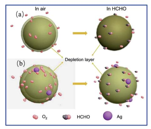
Fig. 37 Schematic model of the depletion layer for SnO<sub>2</sub>/Sn<sub>3</sub>O<sub>4</sub> materials when exposed to air and HCHO (a) before Aq decoration and (b) after Ag decoration, 436 presented with permission and copyright.
