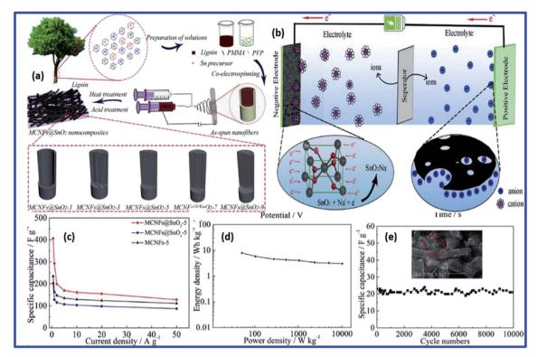
Fig. 33 (a) Fabrication steps for MCNFs@SnO<sub>2</sub>, (b) proposed charge-storage mechanism, (c) current density vs. specific capacities for various electrodes, (d) Ragone plot, and (e) cyclic performance of symmetric capacitors of MCNFs@SnO<sub>2</sub>-5 at 1 A  $g^{-1}$  (inset: SEM image of MCNFs@SnO<sub>2</sub>-5),<sup>406</sup> presented with permission and copyright.
