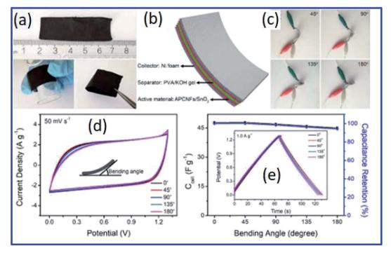
Fig. 34 (a) Flexible APCNFs/SnO<sub>2</sub> membrane, (b) sandwich-type symmetric cell, (c) optical image, (d) CV curves and (e) specific capacitance and capacity retention at various bending angles (inset: their corresponding galvanostatic charge–discharge profiles),<sup>410</sup> presented with permission and copyright.
