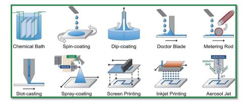
Fig. 4 Various solution-based approaches for metal oxide film deposition. Reproduced with permission. 139 Copyright 2011, The Royal Society of Chemistry.
