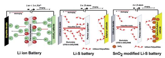
Fig. 31 Schematic of conventional LIBs, Li-S batteries and SnO<sub>2</sub> modified Li-S batteries.
