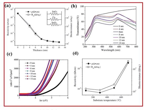
Fig. 8 (a) Resistivity and sheet resistance of  $SnO_2/Cu/SnO_2$  multilayer films deposited at 500 °C as a function of Cu layer thickness. (b) Optical transmittance of  $SnO_2/Cu/SnO_2$  multilayer films deposited at 500 °C. (c) The  $(\alpha h \nu)^2$  relation for  $SnO_2/Cu/SnO_2$  multilayer films. (d) Sheet resistance and resistivity of  $SnO_2/Cu/SnO_2$  multilayer films developed at different substrate temperatures, presented with permission and copyright.
