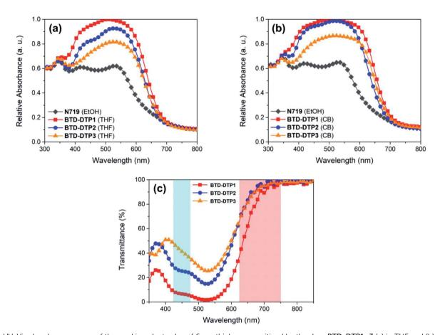
Fig. 5 UV-Vis absorbance curves of the working electrodes of 6 µm thickness sensitized by the dyes BTD-DTP1-3 (a) in THF and (b) in chlorobenzene (CB) solution and, for comparison, by N719 in ethanol (EtOH) solution, obtained from DRS experiments. (c) Transmittance spectra of thin (5  $\mu$ m) transparent TiO<sub>2</sub> films stained with THF solutions of dyes BTD-DTP1-3. Photosynthetically active regions are coloured in cyan (425– 475 nm) and red (625-750 nm).
