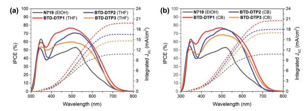
Fig. 7 Solid lines: IPCE curves of the solar cells that employed the working electrodes of 6 μm thickness sensitized by the different dyes. Dotted lines: Integrated short-circuit currents. (a) Sensitization from THF solution; (b) sensitization from CB solution.
