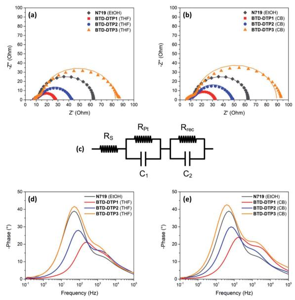
Fig. 8 Nyquist plots (a, b), equivalent circuit used for their fitting (c), and Bode phase diagrams (d, e) for the solar cells that employed the working electrodes of 6 µm thickness sensitized by the different dyes. (a, d) Sensitization from THF solution; (b, e) sensitization from CB solution.
