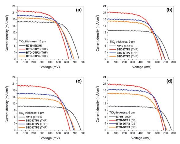
Fig. 6 J-V curves of the solar cells that employed working electrodes of different thicknesses sensitized by organic dyes BTD-DTP1-3 as well as Ru-dye N719. (a) 15  $\mu$ m, THF solution; (b) 9  $\mu$ m, THF solution; (c) 6  $\mu$ m, THF solution; (d) 6  $\mu$ m, CB solution.
